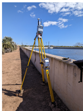
Fig. 6: Experimental setup and location for GNSS Reflectometry testing
